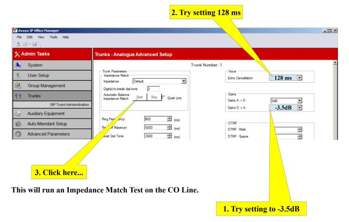
The Gains D-> A is the Audio Level from the KSU to the CO Line. You can try different values to see which works best. This is usually the best way to stop echo.
